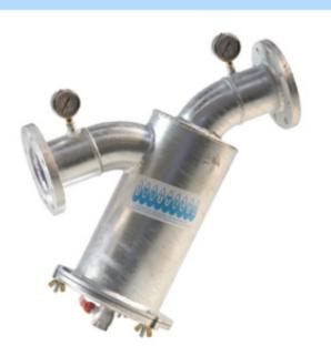
This kind of filter is one of the simplest among the several techniques of filtration and shower installations. It is made of hot galvanized steel, formed by a cylindrical container, which has inside a filtering cartridge of different sieve according to the type of water to filter or to the type of installations, drip or shower.
