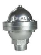
It is used to eliminate air from the underground pipeline and it is positioned on the highest points of the plant. It is made of light alloy with rubber ball.
